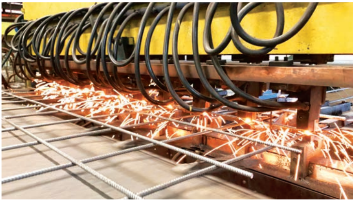
Electric Resistance Welding (ERW)
